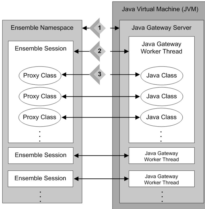
The Java Gateway server runs in the JVM. Ensemble and the JVM may be running on the same machine or on different machines. The items (1), (2), and (3) in the preceding diagram represent the relationships established by the commands that set up this operational model:
